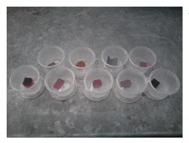
Small samples of each tested filter were taken for microscopic analysis.
