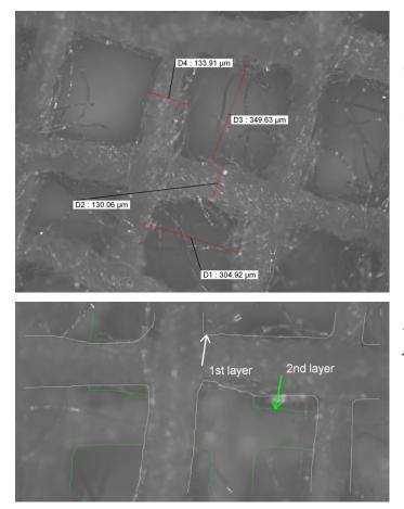
The DNA filter element is another of the woven cotton elements, again consisting of multiple offset layers, in this case 4.
