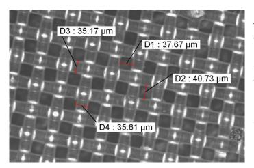
Sprint Filter, SFP08 WP (Water Proof), single layer polyester based element, "Treatment applied to original P08 Material to reduce weave area resulting in waterproof material due to surface tension of water".
