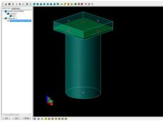
The same test rig which was used for the flow bench tests has been imported into wave from the original NX drawings, and will be used as the main inlet into the engine. The green element seen here is representing a flattened piece of test material.
