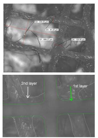
K&N also uses a cotton based woven fibre, like BMC its road filter uses 4 offset sheets of this material.
