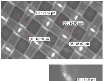
Increased zoom by 10x for SFP08 analysis, Uniformity in weave is apparent from these images. Lack of defects and no requirement to offset layers.
