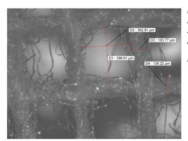
Identical woven cotton construction to its race counterpart however consists of 4 offset layers to increase filtration at a cost of overall flow.
