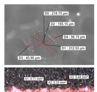
Pipercross is the second of the sponge based elements that was tested, it is made up by 2 layers of sponge.
