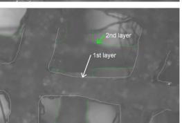
K&N's Race filter is similar to that of the BMC, consisting of 2 offset woven cotton layers. The definition between race and road for many of these filters is simply a reduction in layers.
