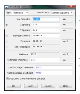
It is easy to see how the filter characteristics of the single element filters could be imported into the Wave model. The process becomes increasingly more difficult with each layer of material added. As the layers are not uniformly offset with most of the multilayer type filters, it becomes increasingly more difficult to simulate the air flow accurately through them.
